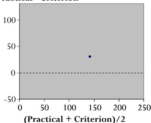
Here is the start of a Bland-Altman plot, which is supposed to tell you all about the interchangeability of two measures. Up the vertical axis you put the difference between the measures, and on the horizontal axis you put their mean. I've dotted in zero difference, which is the ideal result for interchangeability. And now here are our previous data:
